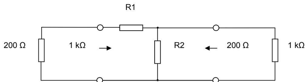
It makes the calculations clearer if we work in kilohms, so that 1 kΩ appears as '1' and 200 Ω appears as '0.2'. Applying Ohm's Law at the output, we force the output source resistance to be 1 kΩ:
