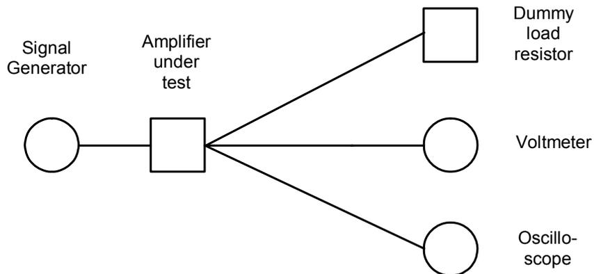
**Figure 1 Test set-up for measuring an amplifier**
