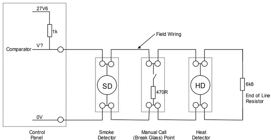
The 1 k $\Omega$  and 6.8 k $\Omega$  resistors form a voltage divider and in the quiescent condition the voltage measured by the comparator at point V? is approximately 24 V. When a manual call point is operated, the switch latches mechanically and connects the 470  $\Omega$  resistor in parallel with the 1k ohm resistor. This equals about 440 ohms so the comparator measures about 8.4 Volts at V?, and causes the alarm to sound.
