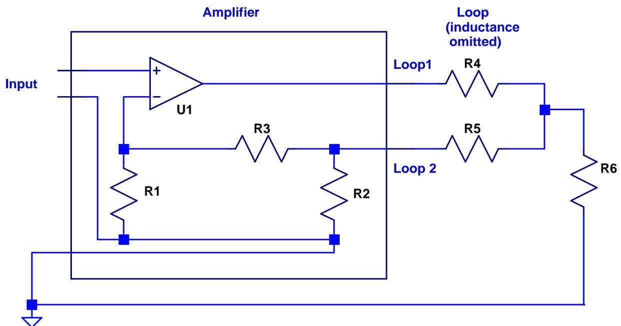
**Figure 1 Amplifier and loop showing an earth fault at the junction of R4, R5 and R6**
